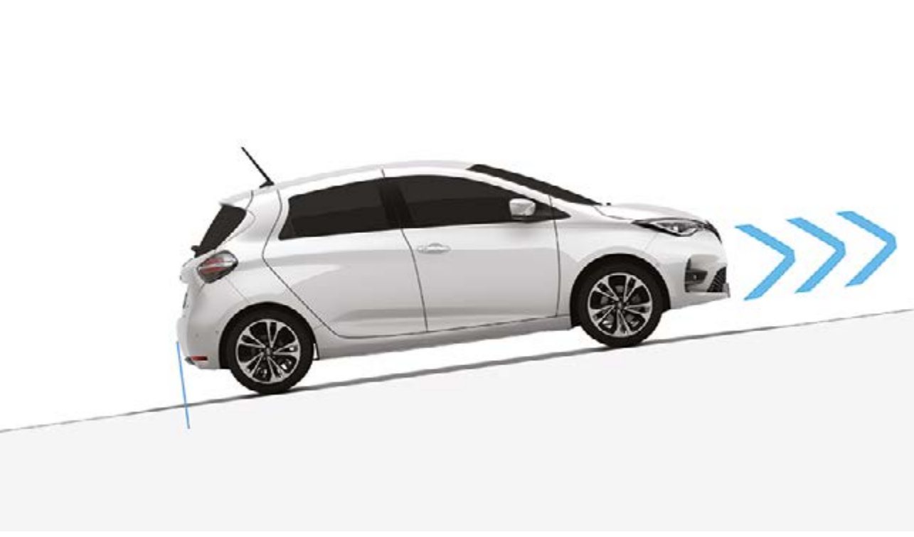
hill start assist Combined with electronic stability control, hill start assist maintains brake pressure automatically for 2 seconds to give you time to lift your foot from the brake pedal and press the accelerator. The system activates when the slope exceeds 3%.
